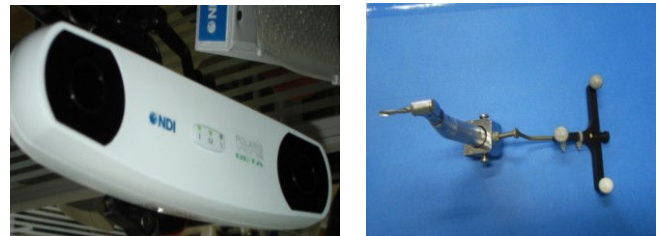
Fig.12 Optical tracker(left) and surgical instrument with spheres(right)
